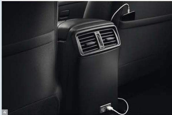
4- CHARGING DOUBLE USB SOCKET FOR SECOND ROW - KE930-HV501
